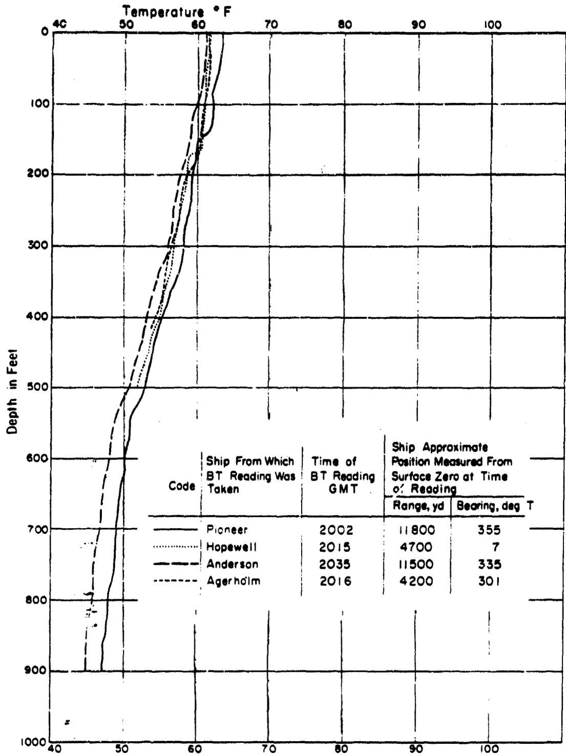
Figure 4.3 Bathythermographs near shot time at various ship positions.
